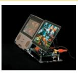
Kodak's active matrix OLED screens offer brilliant, saturated color with high contrast for better perceived sharpness. And the high-speed refresh rate (1000X faster than LCD) adds crispness and clarity to fullmotion video.
